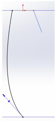
Second, end the spline at the point drawn in the center of Plane 2 then hit the "Escape" key. Feel free to manipulate the shape of this spline as you did with the first spline. Then, Exit Sketch.
