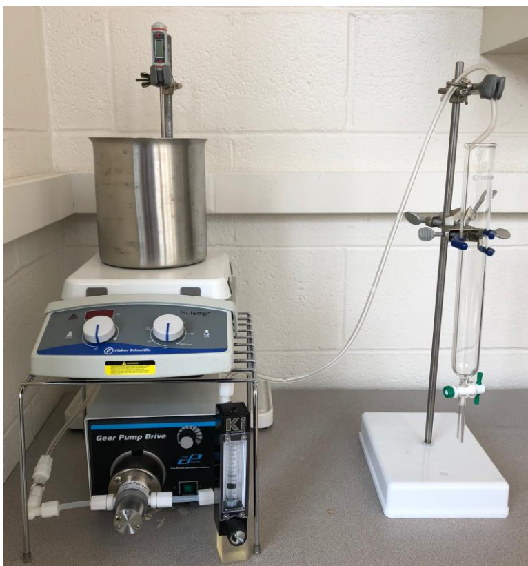
Figure 1. Solid-Liquid Extraction Set Up. Hot water bath and flowmeter connected by a gear pump drive.
